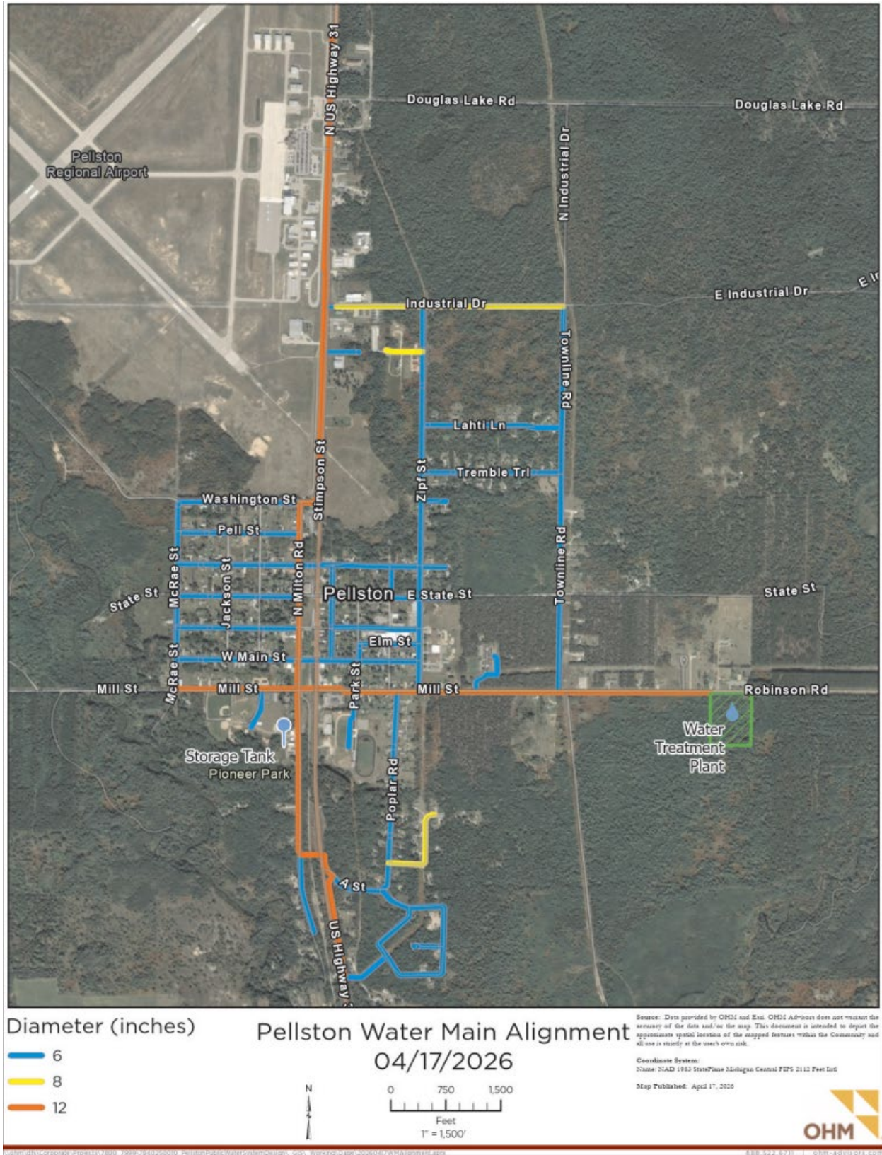
Figure 2: Municipal Water System Layout
